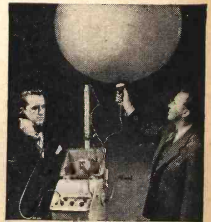
Joseph McDonald and Donald Kolb (holding balloon) are the Radiomarine engineers who developed this lifeboat radio. Here is the balloon that is inflated with helium and carries the antenna as high as 300 feet into the air.
